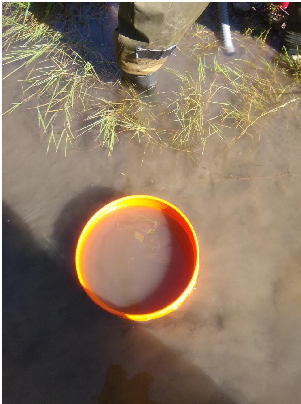
Figure D.5. Lambert and Walling (1998) method for fine sediment collection for the flume experiments.
