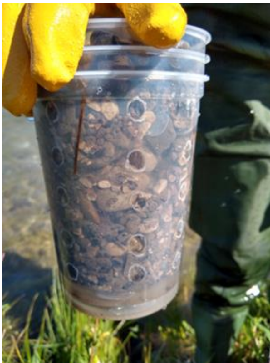
Figure B.3. Example of a sediment trap, designs HV and H (deployed with a lid).
