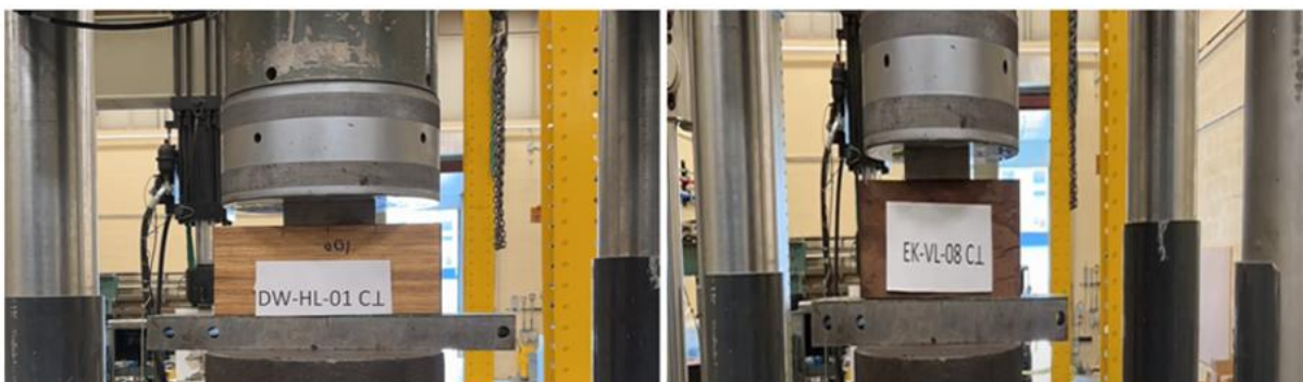
Figure 3.5: Images of Dragonwood and Ekki Specimens under compression perpendicular to grain test set-up
