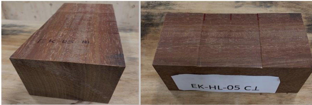
Figure 4.16: Images from failure during compression tests (Ekki beams; horizontal orientation)
