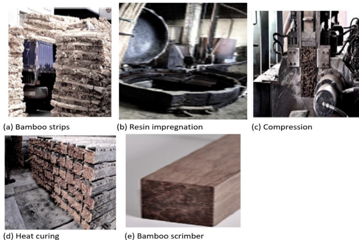
Figure 2.4: Manufacturing process of Bamboo Scrimber
