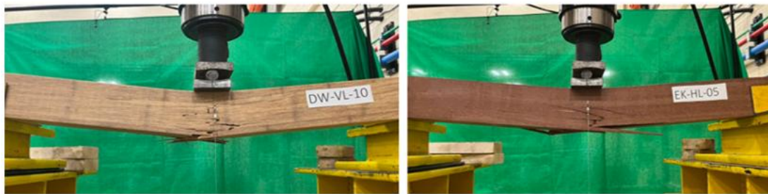
Figure 4.1: Dragonwood and Ekki beams tested under static test set-up
