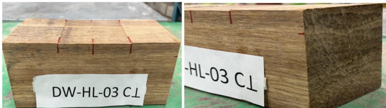
Figure 4.14: Images from failure during compression tests (Dragonwood; horizontal orientation)
