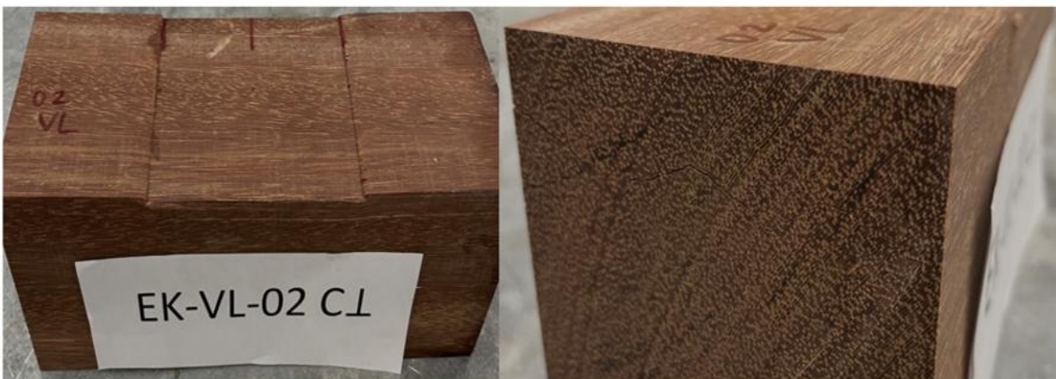
Figure 4.17: Images from failure during compression tests (Ekki beams; vertical orientation)
