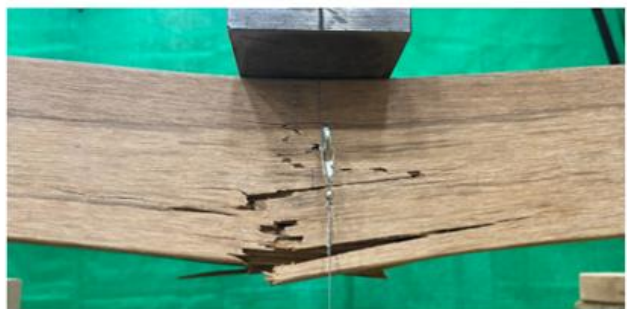
(b) Failure in Dragonwood
