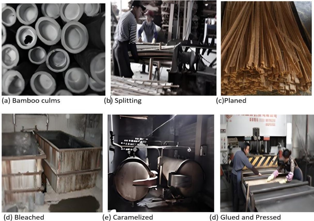
Figure 2.6: Manufacturing process of laminated bamboo
