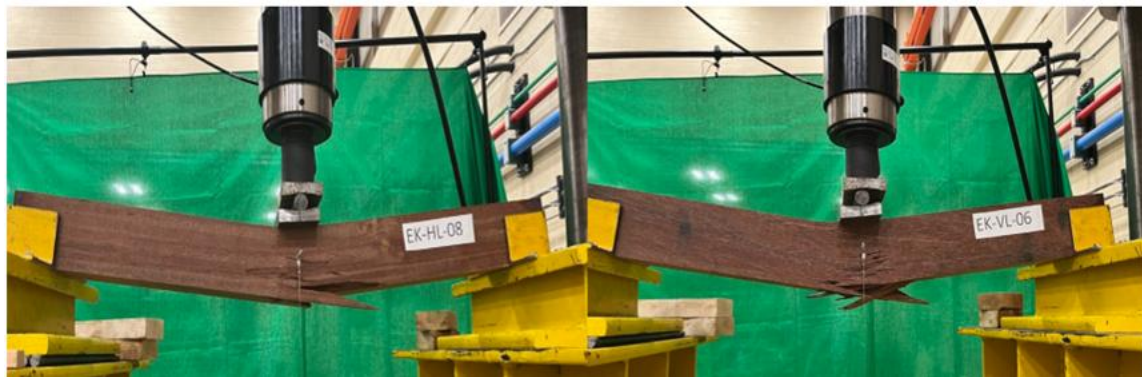
Figure 4.3: Splintering tension failure of Ekki beams in both horizontal and vertical orientations
