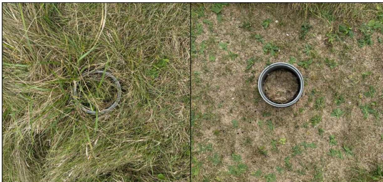
Figure 2.2: Vegetated (Left) and Non-Vegetated (Right) Plots with Installed Collars in the Landfill Cover Soil
