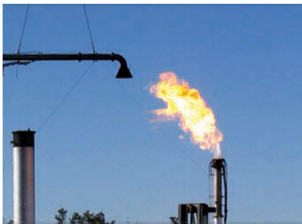
Figure 2: Even in the case of full-scale validation experiments, the CE or DRE of the flare is connected to the measurements (plume gas composition) by an instrument model derived from assumptions and simplifications, e.g., that the sampled gases represent the overall flare emissions [23].
