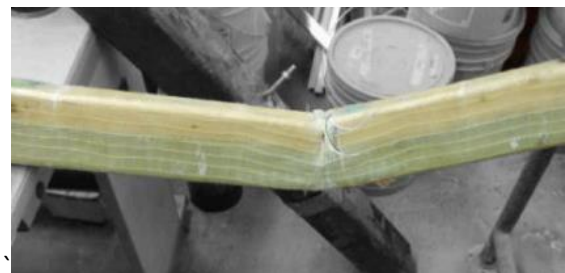
(b) Full confinement failure (localized damage)
