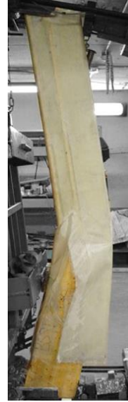
(b) Unzipping failure
