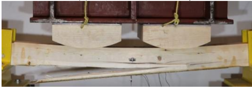
(c) Failure at FRP termination point
