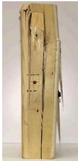
(a) Unreinforced member failure
