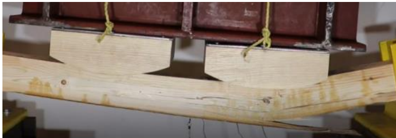
(b) Failure at FRP termination point
