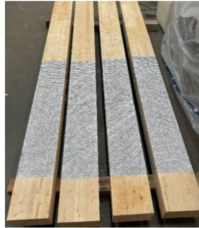
(b) Flexural tests
