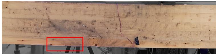
(a) U-01: Initial splintering failure
