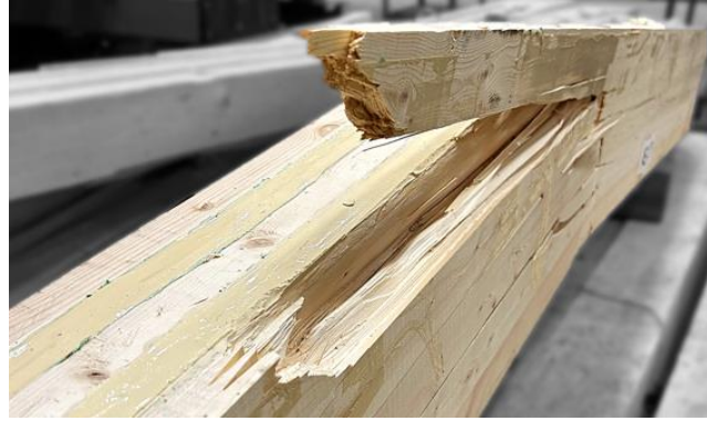
Figure 6.5 Tension failure stemming from edge (R2-3)
