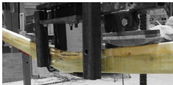
(a) U-shaped failure (localized damage)
