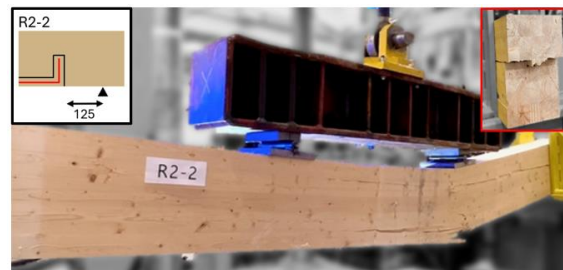
Figure 4.20 Initial shear failure followed by simple tension of beam R2-2
