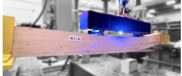
(6) Failures continue to propagate
