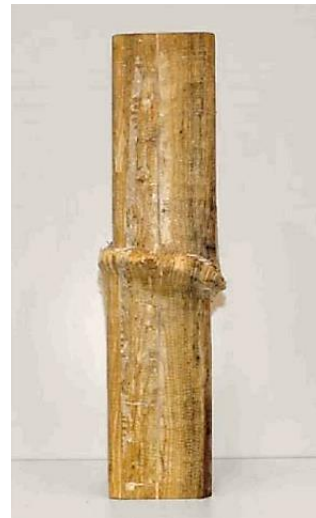
(b) GFRP-reinforced member failure
