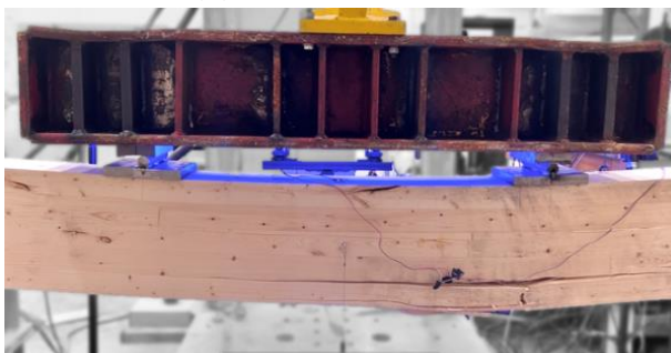
(5) Failures continue to propagate
