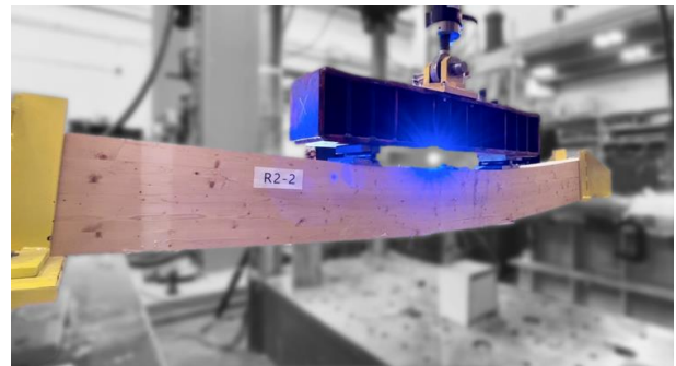
(4) Simple tension failure
