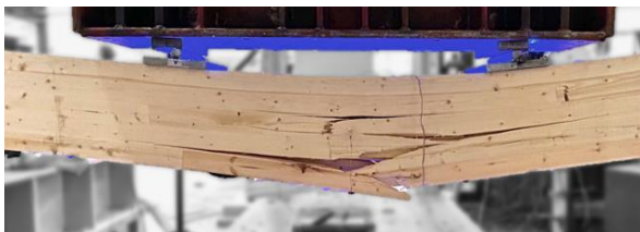
(c) Representative splintering failure (U-04)
