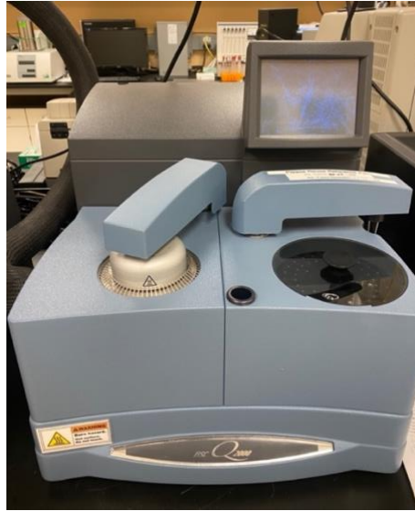
Figure 24 Differential Scanning Calorimetry (DSC)
