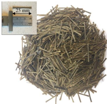
Figure 3 Aramid Fibres Used in the Study
