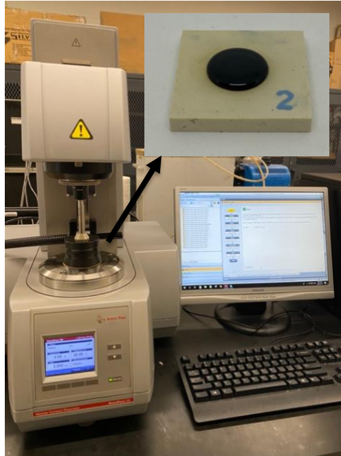
Figure 25 Dynamic Shear Rheometer (DSR) Test set-up
