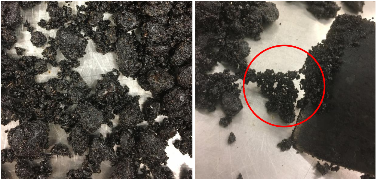
Figure 4 Loose Mixture with Fibres Before Compaction
