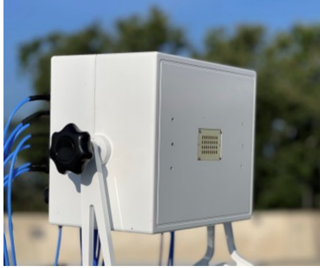
Fig. 2.4: Fully digital beamforming 32 elements antenna array. [3]
