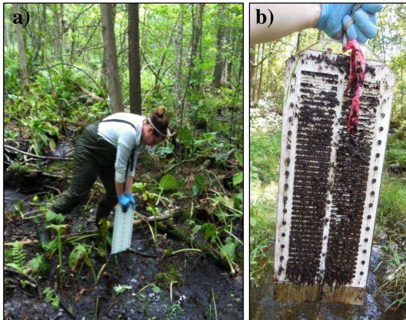
Figure 2-8. a) Deployment of peeper sampling devices into the riparian sediment. b) Removal of peeper from sediment after 28 days.
