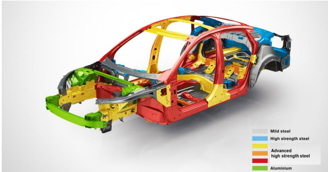
Figure 2.2: Material distribution in the body structure of Volvo XC90 [29]
