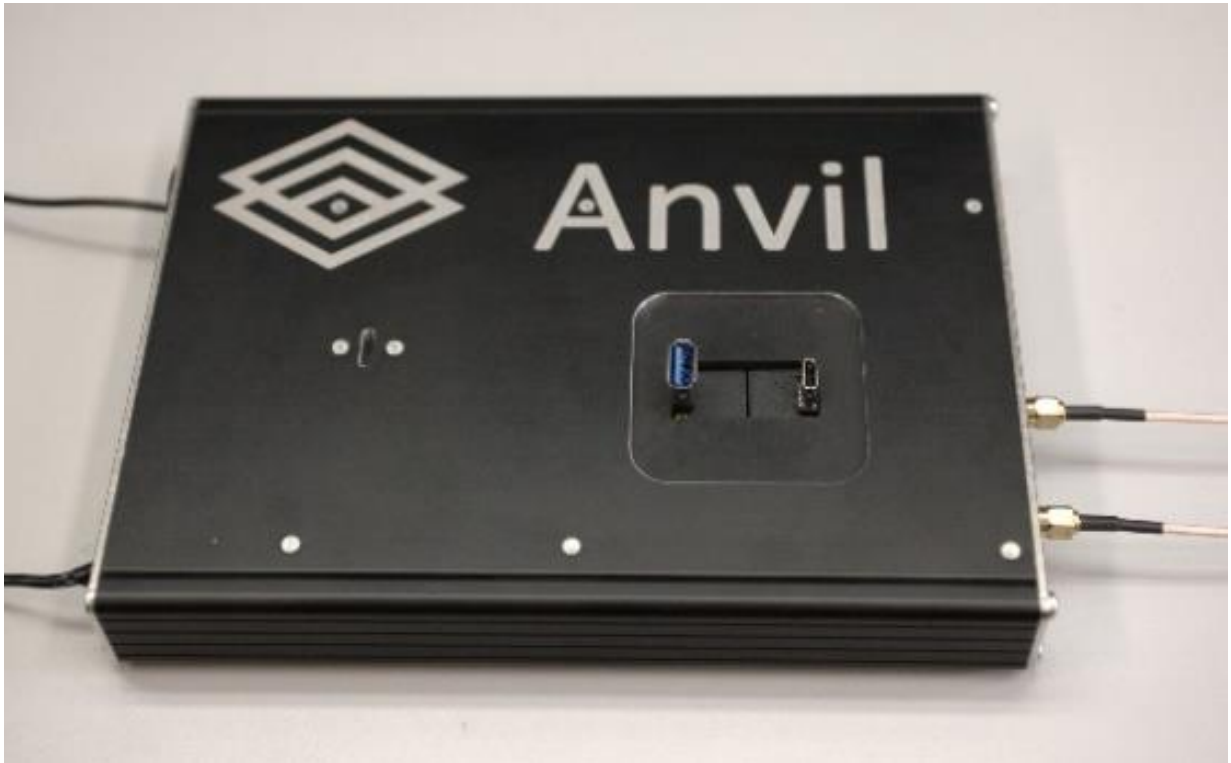
Figure 2.1: A photo of the SILGEO measurement device with a USB adapter board. Note that SILGEO was rebranded to Anvil, hence the label seen in the photo. (This photo was taken by Srijan Pabbi)
