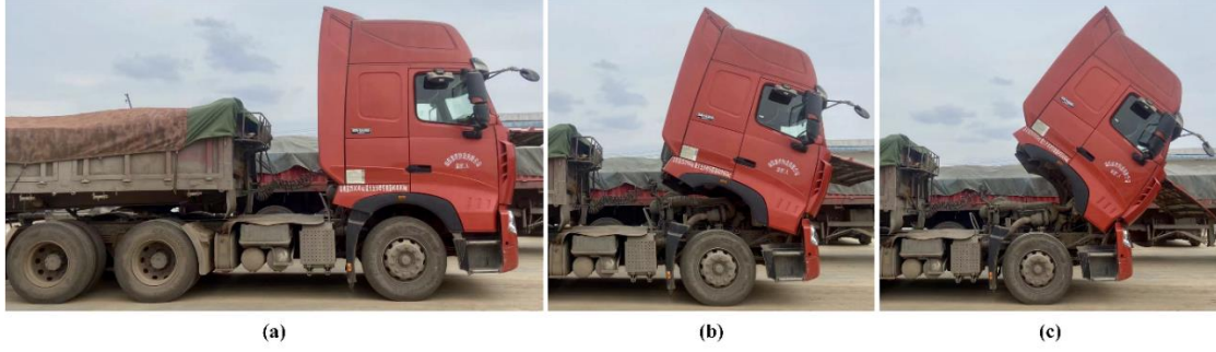
Figure 3.1. Cabin tilting of a flat-nose truck
