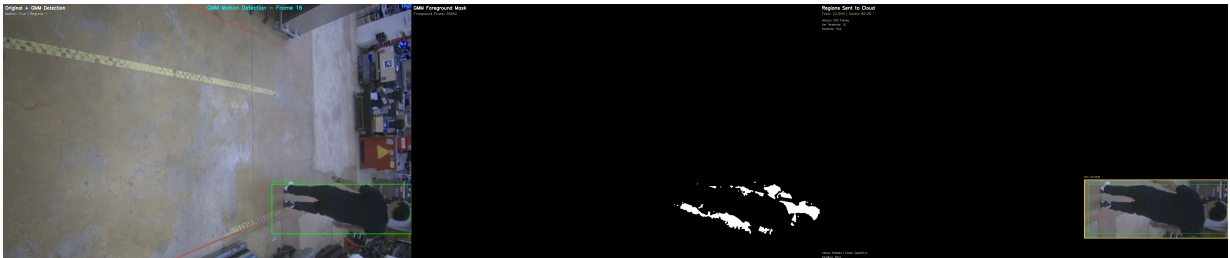
Figure 6.2: GMM three-panel visualization showing: (left) bounding boxes on input frame, (center) motion mask from background subtraction, (right) compressed regions transmitted to cloud.
