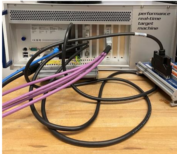
Figure 33 : Speedgoat Performance Unit Injecting Open Loop Testing Data for HIL Testing
