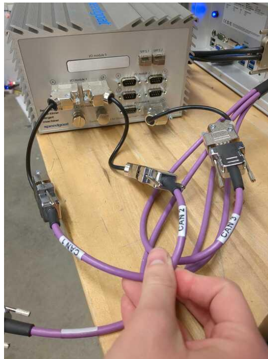
Figure 34 : UWAFTHIL Setup with Speedgoat Unit Communication
