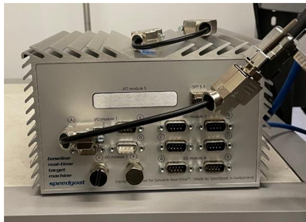
Figure 32 : Speedgoat Baseline M Controller Running Control Logic for HIL Testing
