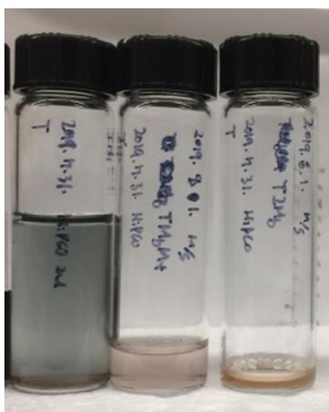
Figure 4.18: Simple process sorting results with HiPCO SWNTs.
