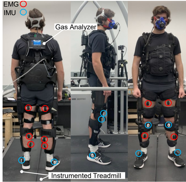
Figure 5.2: Dorsal, lateral, and frontal view of a participant with the Indego exoskeleton with active hip and knee joints. The participant is standing on the Bertec treadmill with two speed-controlled belts equipped with individual loadcells underneath each of them for GRF monitoring. Muscle activation is measured from both right and left leg muscles using EMG sensors. Gait up IMUs are clipped to the outer side of the shoes right bellow ankle joints to measure the spatiotemporal parameters of gait. Oxygen uptake of the participant is measured and recorder at each breath through a mask connected to the gas analyzer device carried at the back of the participant.
