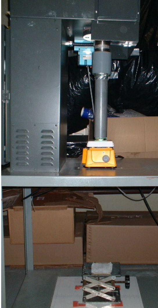
Figure C.2 LP or MP UV Bench-scale collimated beam apparatus (left: a shorter beam; right: a longer beam)
