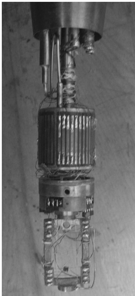
Figure 3.9: A close-up of sample holder along with 1K pot
