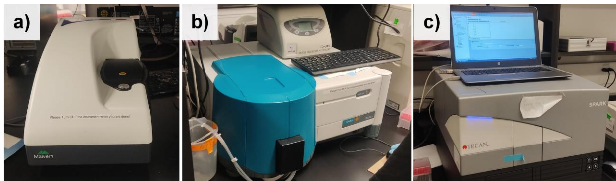
Figure 2.7. A collection of characterization equipment used in this work from Prof. Juewen Liu's Lab in the Chemical Engineering Department at the University of Waterloo: a) Malvern Zetasizer Nano ZS Dynamic Light Scattering device, b) Agilent Cary Eclipse fluorescence spectrophotometer, c) Tecan Spark multimode microplate reader.
