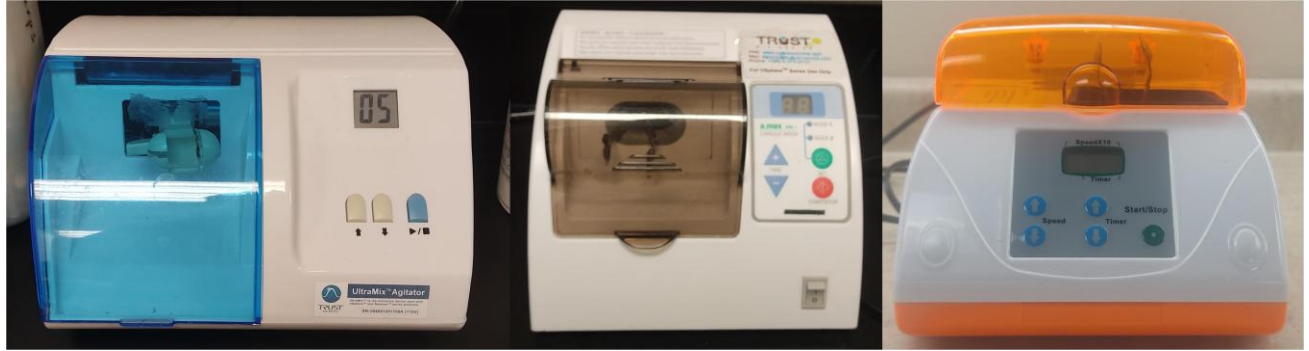
Figure 2.4. Examples of dental amalgamators used to form MBs through mechanical agitation. Two commercial amalgamators sold for TRUST Biosonic bubbles are pictured and operate at a static 4.4kHz. An amalgamator purchased from Amazon with adjustable shake rates. We chose a shake rate of 4.4kHz to be consistent with the commercial bubbles used at our lab.
