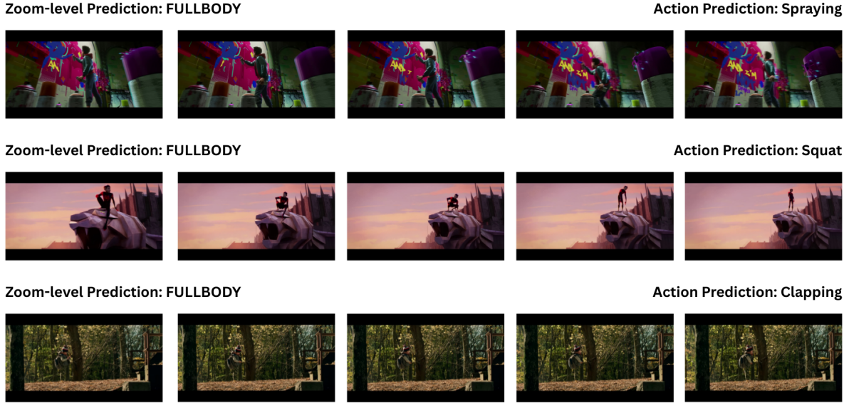
Figure 5.9: Qualitative results of full-body action recognition using STGCN++ pretrained on Kinetics-400. Examples demonstrate correct predictions for spraying and squatting, as well as a misclassification where a boy holding a toy was incorrectly predicted as clapping.
