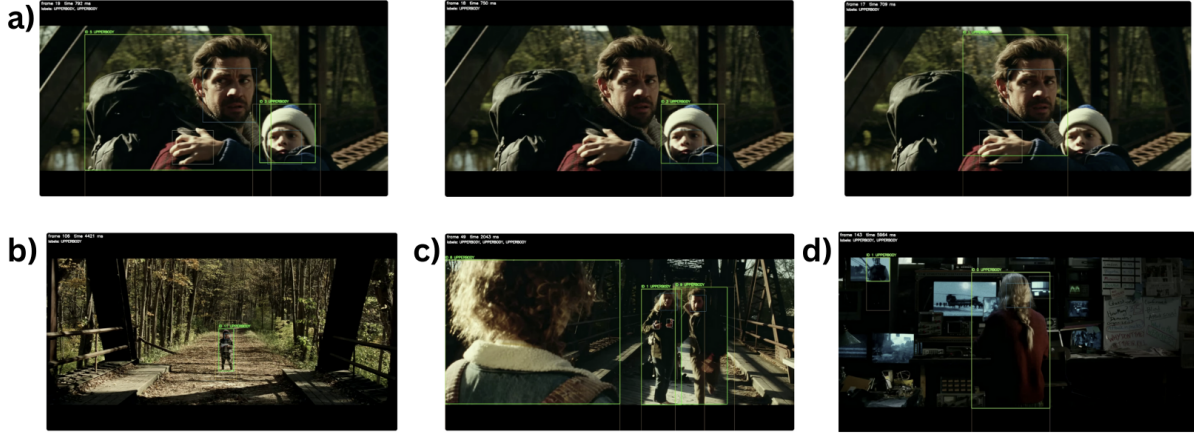
Figure 5.4: Representative failure cases that motivated updates to the heuristic rules. (a) Tracker ID switching across consecutive frames, leading to inconsistent view assignments. (b) Far-scale character misclassified as UPPERBODY instead of FULLBODY . (c) Foreground occluder causes background torso to be missed and misclassified as NOPARTS . (d) Over-sensitive knee detection results in unstable toggling between UPPERBODY and FULLBODY .
