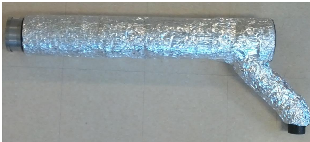
Figure A9- The 10.2cm diameter ABS header covered in insulation to minimize thermal losses.
