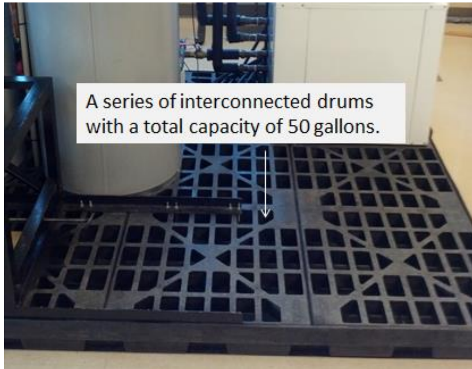
Figure A10- Containment platforms installed beneath the test apparatus to prevent water spillage onto the floors.
