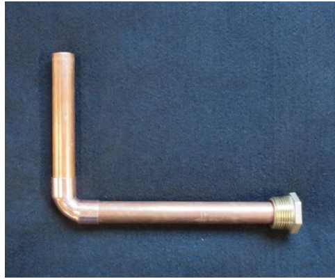
Figure A6- Diagram of the water flow in Cold Tank 1, and the modified pipe used to direct the cold water from the chiller to the very top of the tank.
