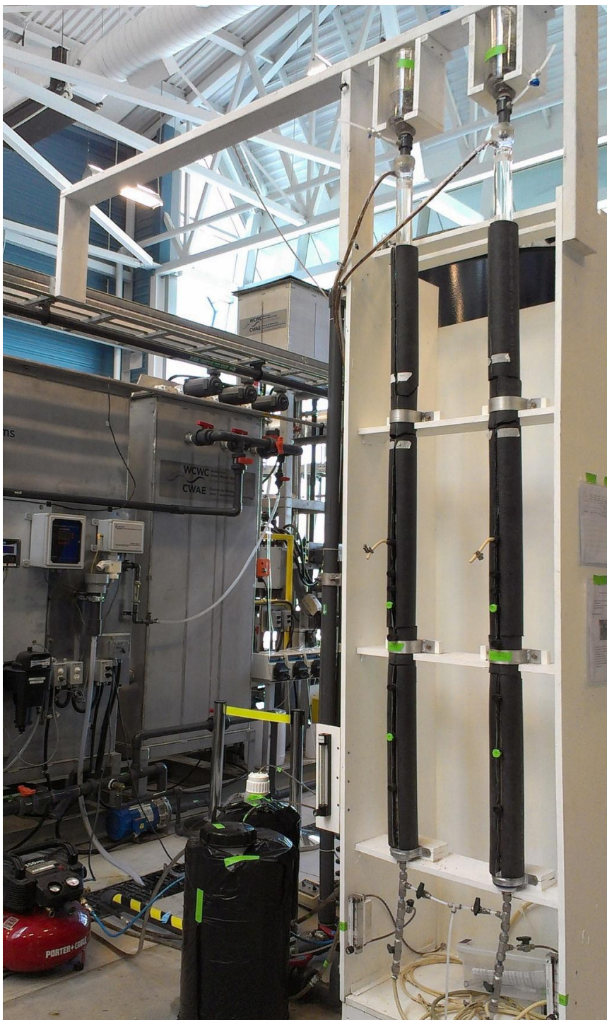
Figure A-5: Biofilter set-up with backwash tanks and backwash air compressor
