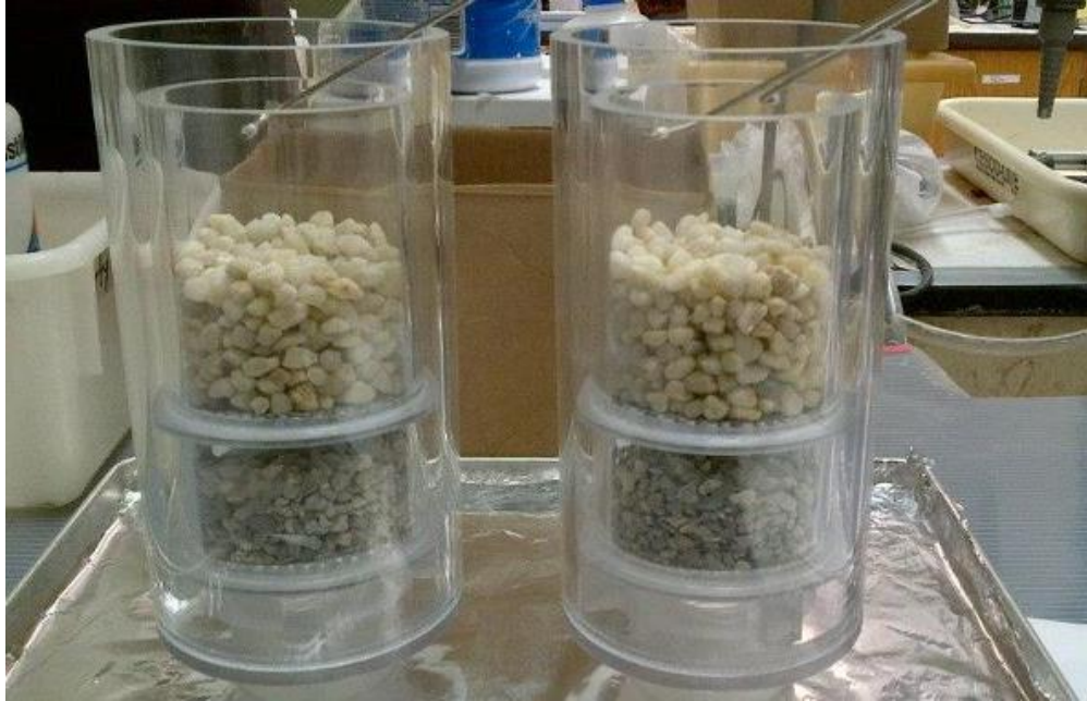
Figure A-3: Roughing filters with gravel as media
