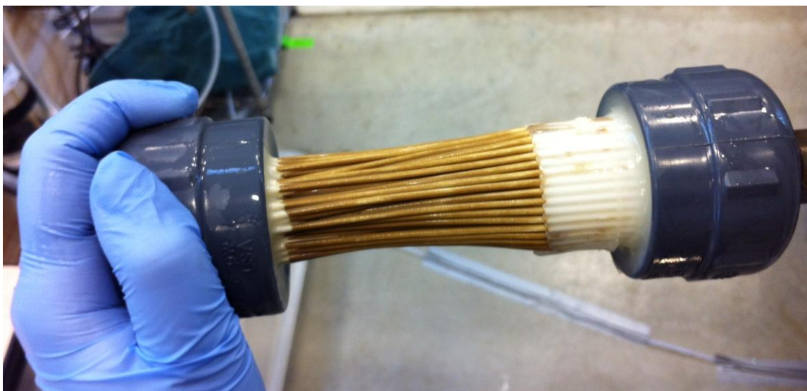
Figure A-13: Fouled membrane unit before chemical cleaning
