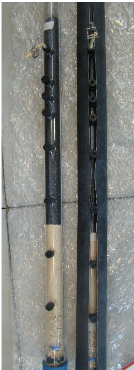
Figure A-2: Fresh sand and anthracite media in the glass columns
