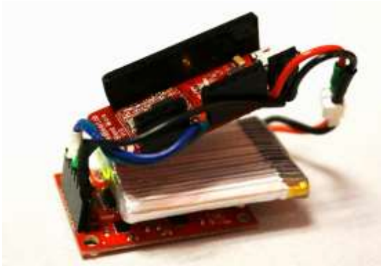
Figure 5. A Blend Micro board, IMU, and battery.
