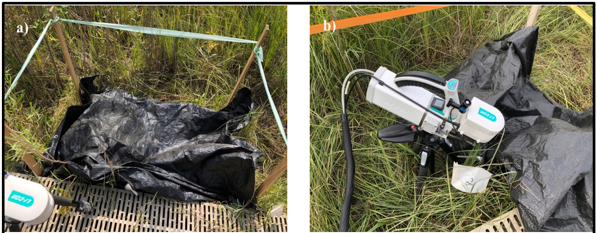
Figure 2-4. Photos of the overall set-up for the dark-adapted measurements. a) The photo demonstrates how each plot was dark-adapted using a black tarp for at least 30 minutes prior to beginning any measurements. b) The photo demonstrates how the dark-adapted measurements were conducted by removing the tarp and placing the C. aquatilis stalks within the gasket of the LI-6800, allowing the flash could be initiated through the console.
