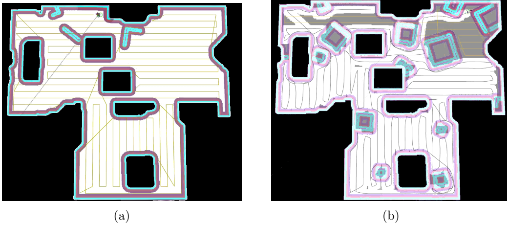
Figure 4.16: Robot operating system (ROS) simulation of covering an example environment with unknown obstacles. (a) An initial coverage path for the base environment (b) replanning the path online using OARP-Replan.
