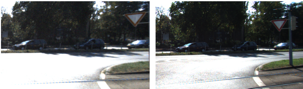
(a) Image from the old camera, where the resolution is lower, the image is noisier, and the field-of-view is narrower. The image also lacks color vibrancy due to low dynamic range.
