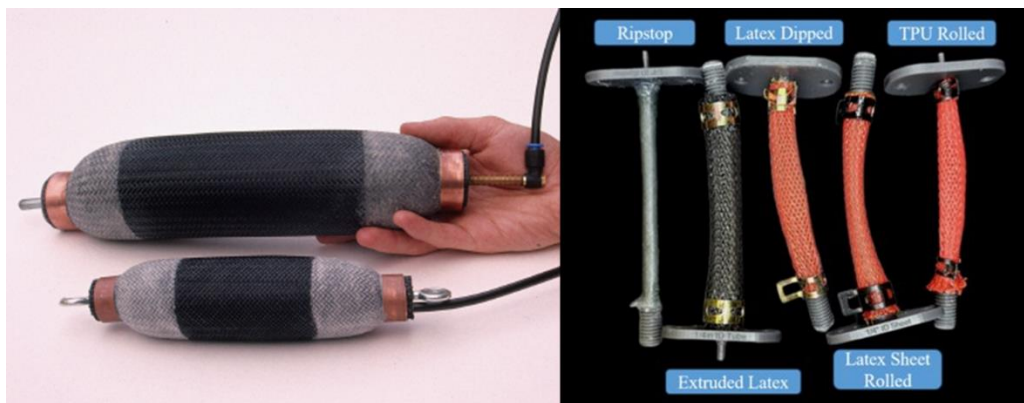
Figure 44. Example of McKibben Artificial muscles and different material constructions. Adapted from [99], [100]
