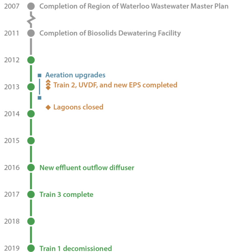
Figure 1.6.1 Broad timeline of upgrades at the Kitchener WWTP adapted from Region of Waterloo (2010). UVDF = UV disinfection, EPS = Effluent pumping station.
