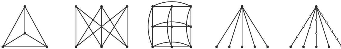
Figure 2: From left to right: the complete graph K_4 , the complete bipartite graph K_{3,3} , the line graph of K_{3,3} , the star K_{1,5} and a subdivision of K_{1,5} .
