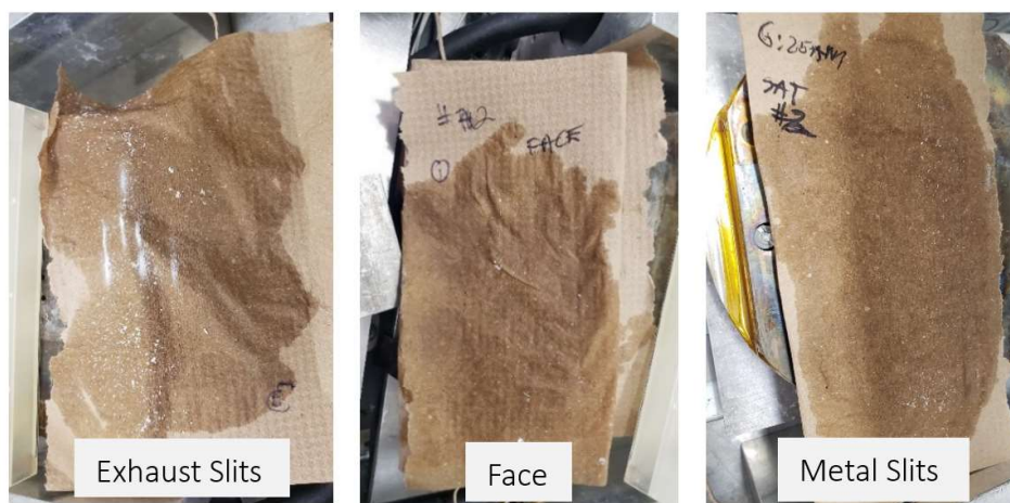
Figure 18: Powder from cleaning different areas of the reactor head. a) Powder found in the exhaust slits. b) Powder found on face of the reactor head. c) Powder found in the metal slits of the reactor head.
