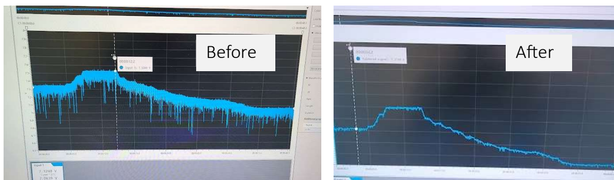
Figure 43: The (pressure) signal before and after maximizing the input voltages to the data loggers. Note how much cleaner the signal is after maximizing the input voltages.
