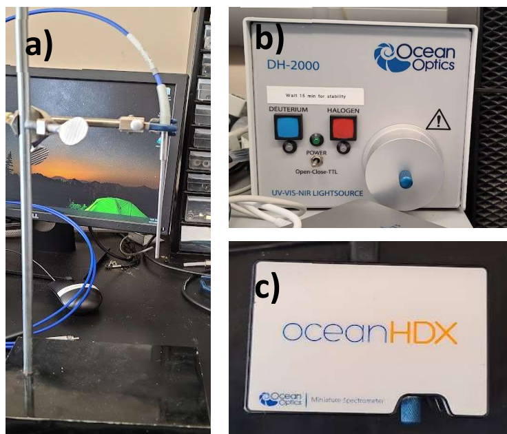
Figure 30: Apparatus used for reflectometry. a) The reflectance probe (EOS-A6177351-2) and stand. b) The DH-200 light source. c) The oceanHDX spectrometer.
