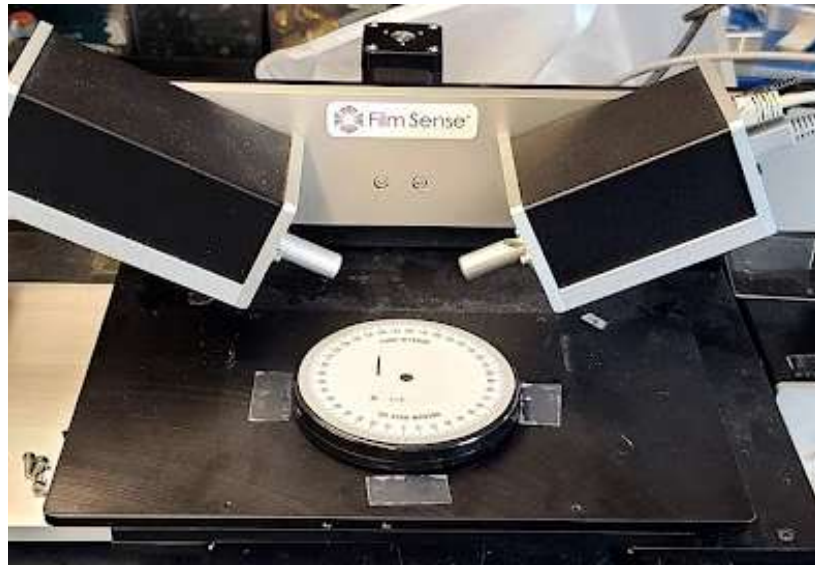
Figure 29: Custom rotary stage used to take ellipsometry data of a sample at different orientations.
