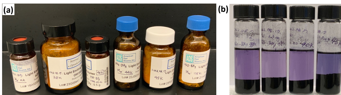
Figure 5.5: (a) A set of PFO-BPy samples with different molecular weights used for dispersion experiments from 33k to 135k g/mol, (b) Resulting dispersions after centrifugation using PFO-BPy samples with molecular weights of 33k, 38k, 40k, and 45k g/mol, respectively.
