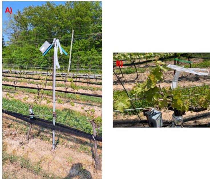
Figure 2-2: A) A TTW sensor deployed to monitor a Cabernet Franc vine at ON_VIN_01, supported by a rod attached to a T-bar used in the trellis system. The battery is positioned above the canopy to keep the solar panel free from vine cover. B) A close-up of the TTW sensor positioned under the canopy.
