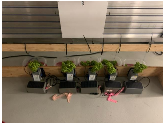
Figure 2-3: A photograph of the rack system that was used to support the grape clusters over top of the TTWs in the Plant Grow Chamber for monitoring grape maturity.
