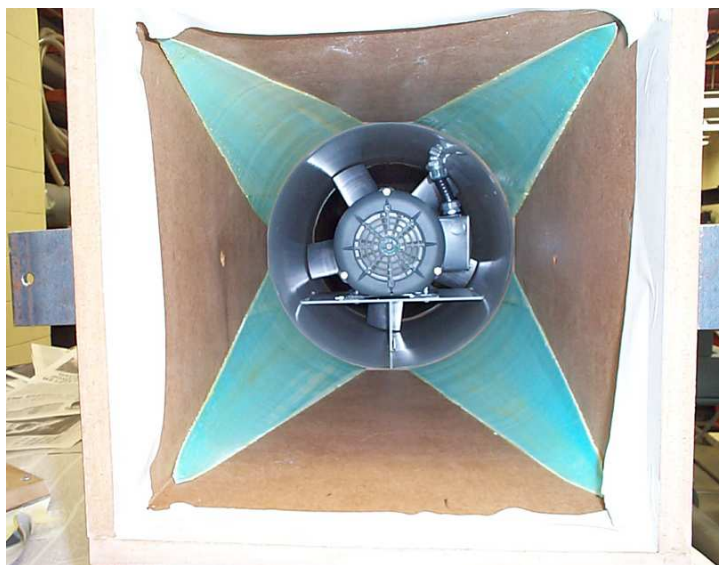
Figure 3.5: Transition 1 with styrofoam filler sections
