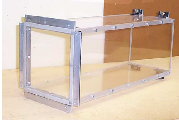
Figure 3.1: Acrylic test section ( 152.4mm \times 152.4mm \times 450mm )
