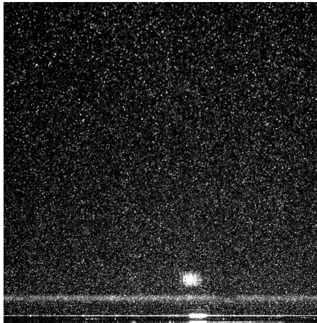
Figure 5.9: Sample PIV image from the test section in the vertical plane (approximate size, 85mm x 85mm , smoke particles in air)
