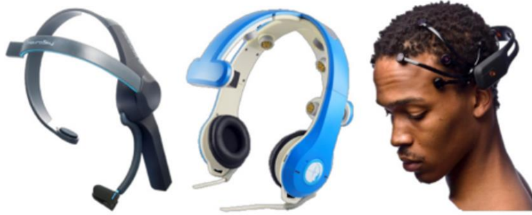
Figure 42. EEG systems with improved convenience: MindWave from NeuroSky, BR8+ from BRI and EPOC from Emotiv (Images [263]).
