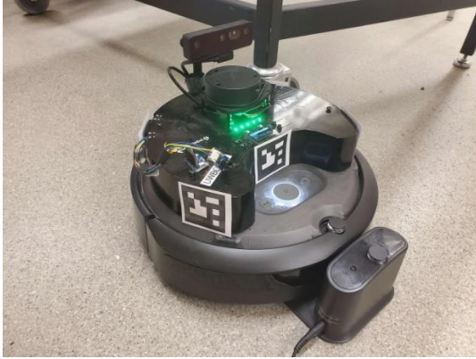
Figure 3.11: Robohub robot with lidar and camera
