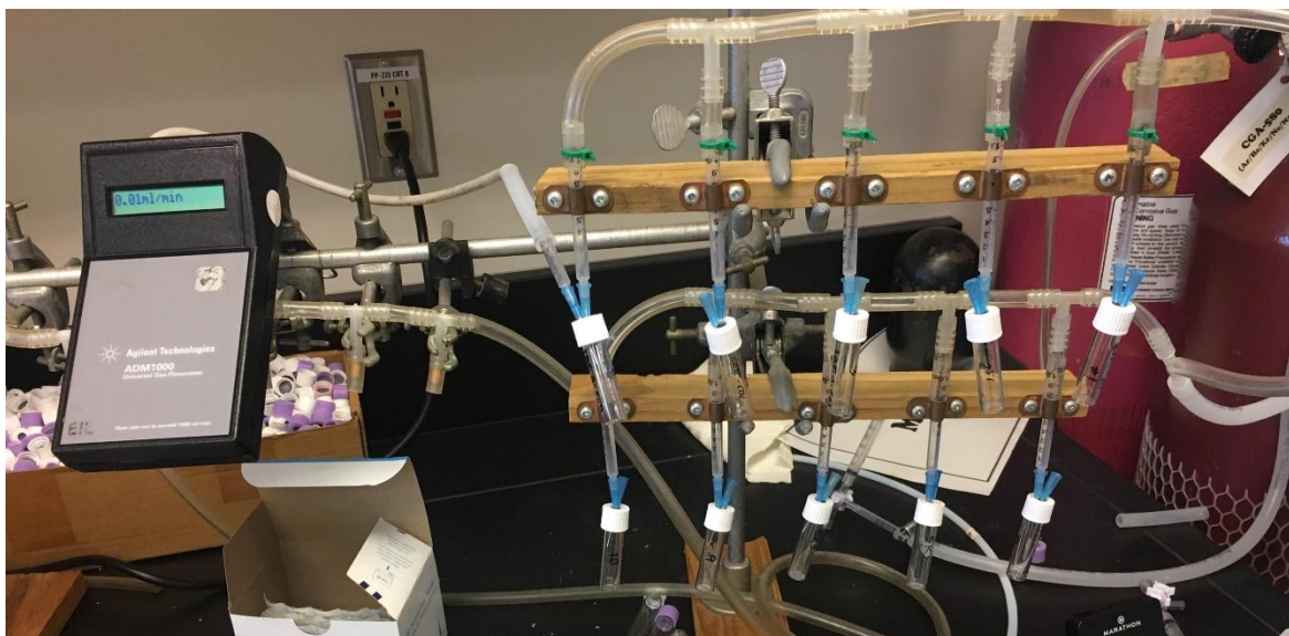
Figure 1. Image of dual-needle gas flushing system at the Environmental Isotope Laboratory (University of Waterloo). Gas flow meter is pictured on the left-hand side, with tubing connecting the meter to the vial through a secondary dispensing needle. Vials are attached to dispensing needle connected to the helium tank.
