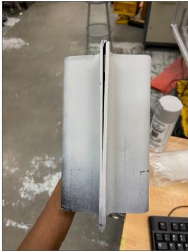
Figure F.2: Debonding of initial [0/\pm 45/90]_s double-hat channel quasi-statically axially loaded.
