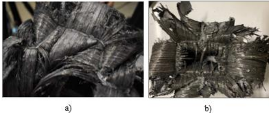
Figure 5.37: Comparison of failure mode of the (a) [\pm 45/0_2]_s hat [25] and (b) [\pm 45/0_2]_s double-hat channels under quasi-static axial loading.
