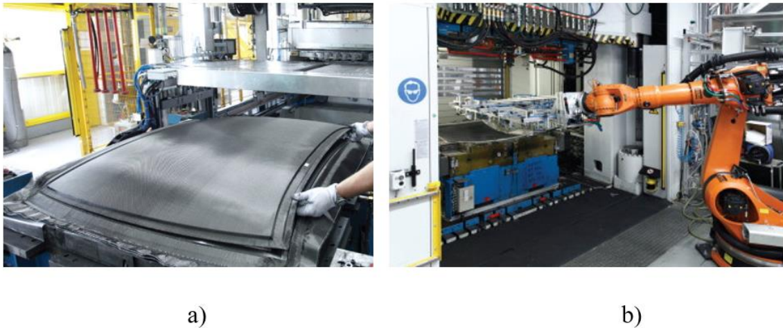
Figure 1.2: (a) Preforming the CFRP roof of the BMW M3 (b) Removal of the BMW M3 roof from a RTM press [10].
