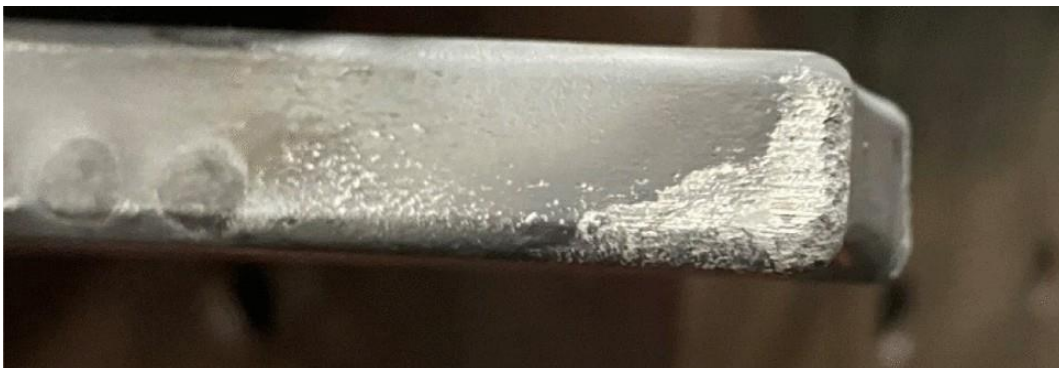
Figure 8: Soldering on a die casting core pin [29]
