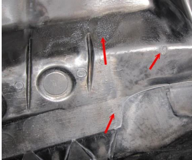
Figure 5: Erosive wear in die [24]
