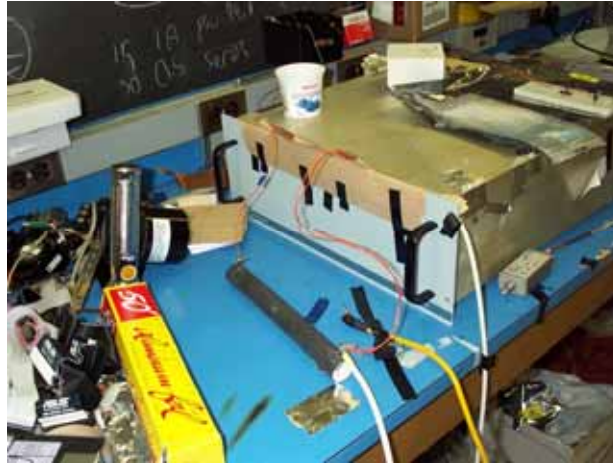
Figure H.1: Lab built modulator packaged in metal enclosure with an external resistor connected
