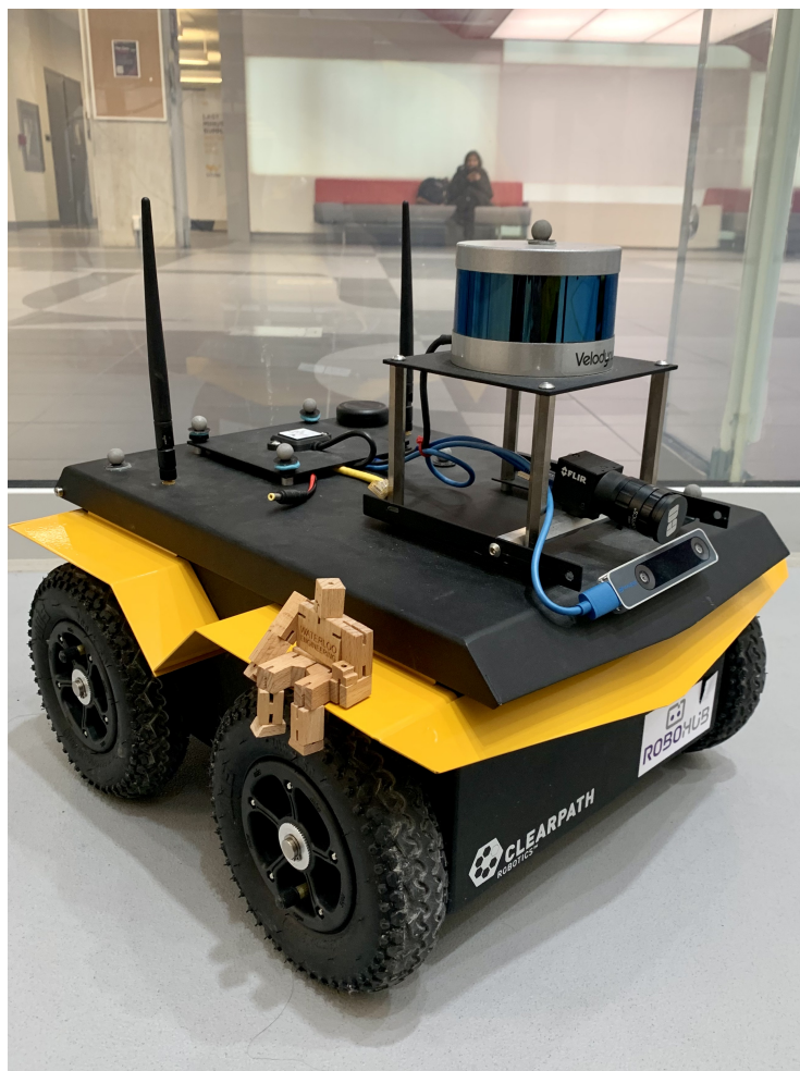
Figure 5.2: A photograph of the Jackal platform used in the study.
