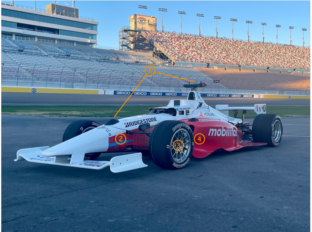
Figure 4.14: Sensor setup for AV-21 during the time-trial. 1. GNSS antennas, 2. steering angle sensor (inside the cabin), 3. wheel encoder (near the axle), 4. INS (inside the cabin).
