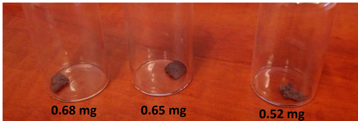
Figure 28: Self-standing electrodes of C-coated SiNW-G
