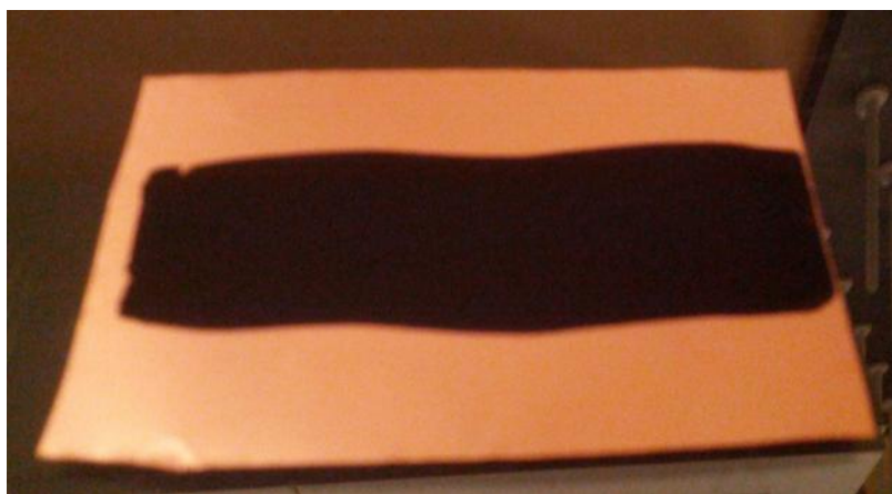
Figure 10: SiNW-G material casted on copper foil with doctor blade
