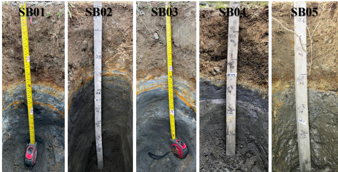
Figure A4. Test pit photos from all sampling locations showing the sand and gravel layer overlying the tailings, with a thin oxidation zone.
