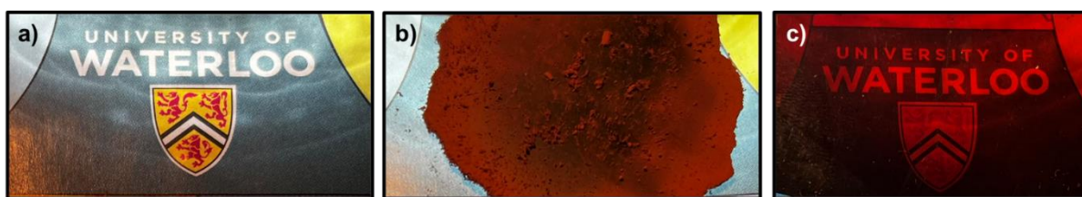
Figure 38. Melt processability and transparency of a) CA film, b) unmodified kraft lignin, and c) esterified lignin samples.
