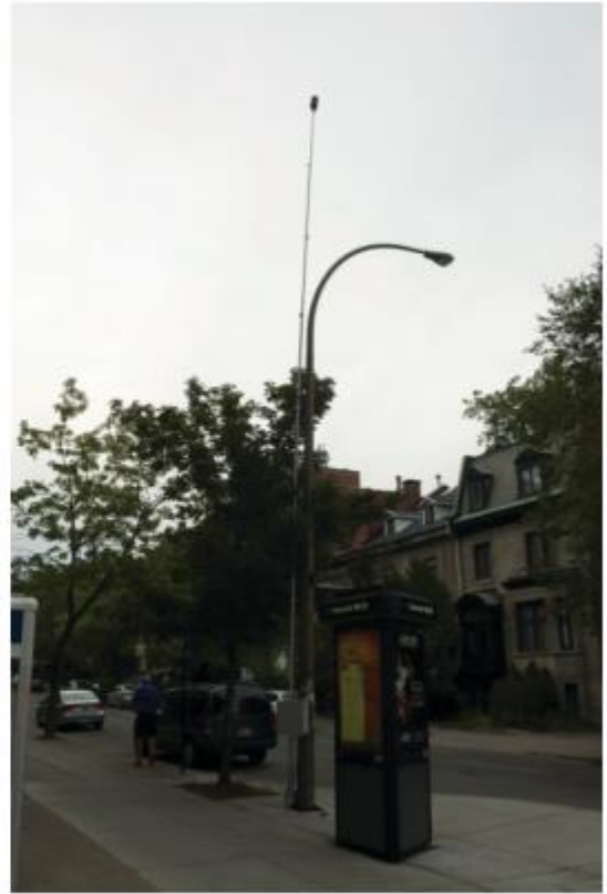
Figure A-1: Mobile video-based traffic conflict analysis system installed in Montreal, Quebec (Jackson et al., 2013)
