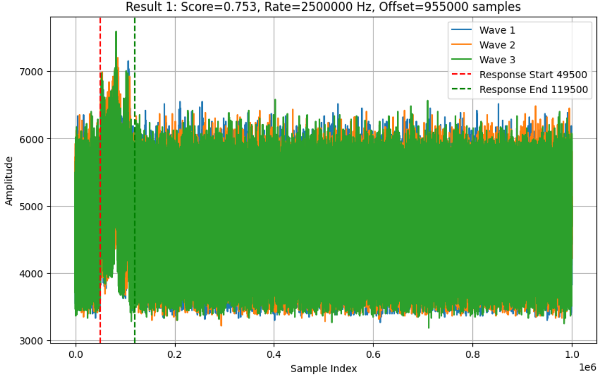
Figure 4.5: Raspberry Pi (SSH): Three representative response traces with the identified response window using optimal parameters
