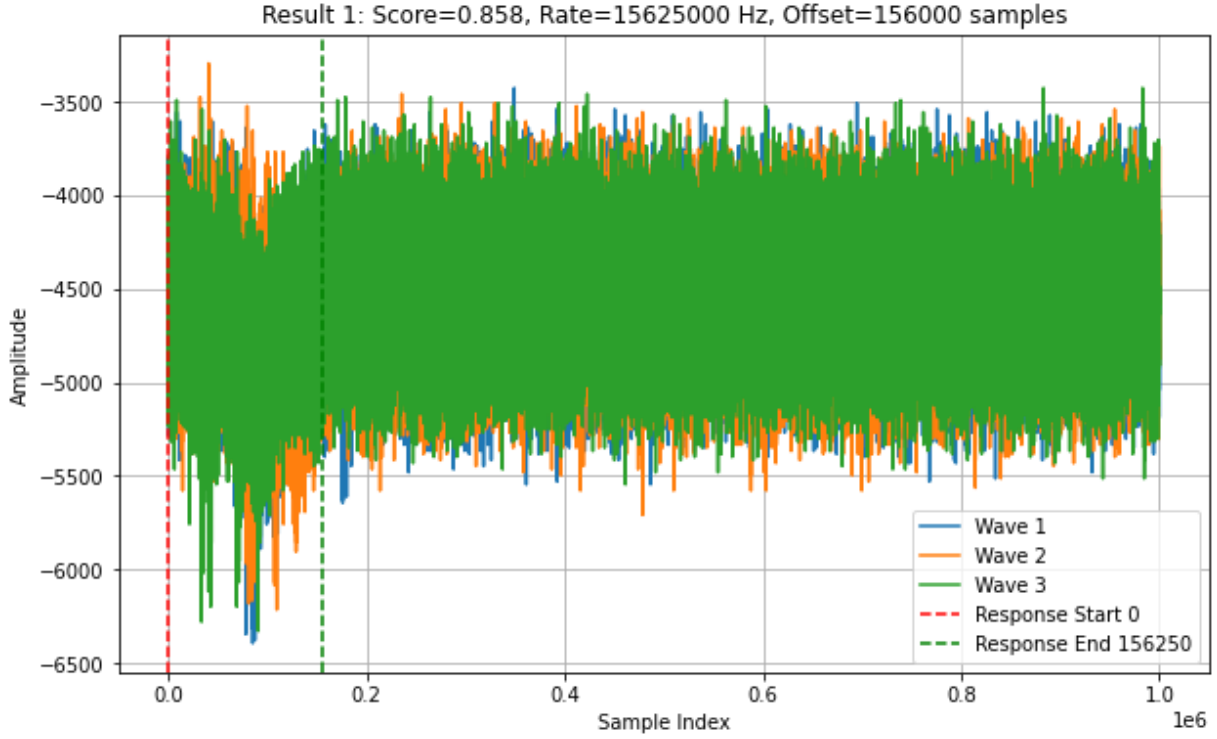
Figure 4.2: OpenEVSE Charger Board: Three representative response traces with the identified response window using optimal parameters
