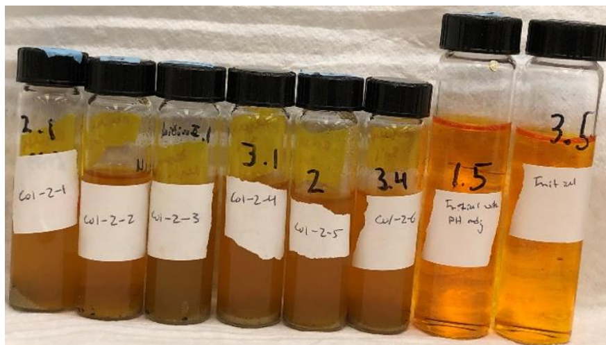
Figure 3.28- An image of the vials used in the tracer analysis of validation set 1, Column 2 samples. All vials contained 100 mg/L Orange G, 100 mM HCOOH, 100 mM HCOONa, and 100 g/L of a validation sample. The vials were labelled with the sample number (e.g., on the far left, Col-2-1). The pH of the solutions in the vials was between 3.6 – 3.7. The first 6 samples from the left contained validation set 1, Column 2 samples, while the 2 vials on the right were control vials, and as such did not contain soil. From left to right: samples Col-2-1, Col-2-2, Col-2-3, Col-2-4, Col-2-5, Col-2-6, and two control vials.
