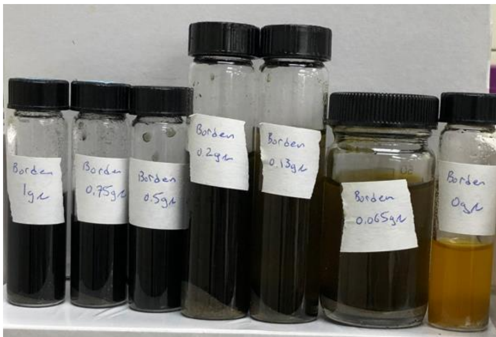
Figure 3.16- An image of the vials used in an experiment with PlumeStop ® -spiked Borden. All vials contained 100 mg/L Orange G, 100 mM HCOOH, 100 mM HCOONa, and 100 g/L of Borden spiked with PlumeStop ® . The concentration of PlumeStop ® ranged between 0 – 1 g/L. The vials were labelled with the soil type present (i.e., Borden) and the concentration of PlumeStop ® (e.g., on the far left, 1 g/L). The pH of the Borden systems in experiments with PlumeStop ® was between 4.5 – 5.9. From left to right: samples with 1, 0.75, 0.5, 0.2, 0.13, 0.065, and 0 g/L of PlumeStop ® .
