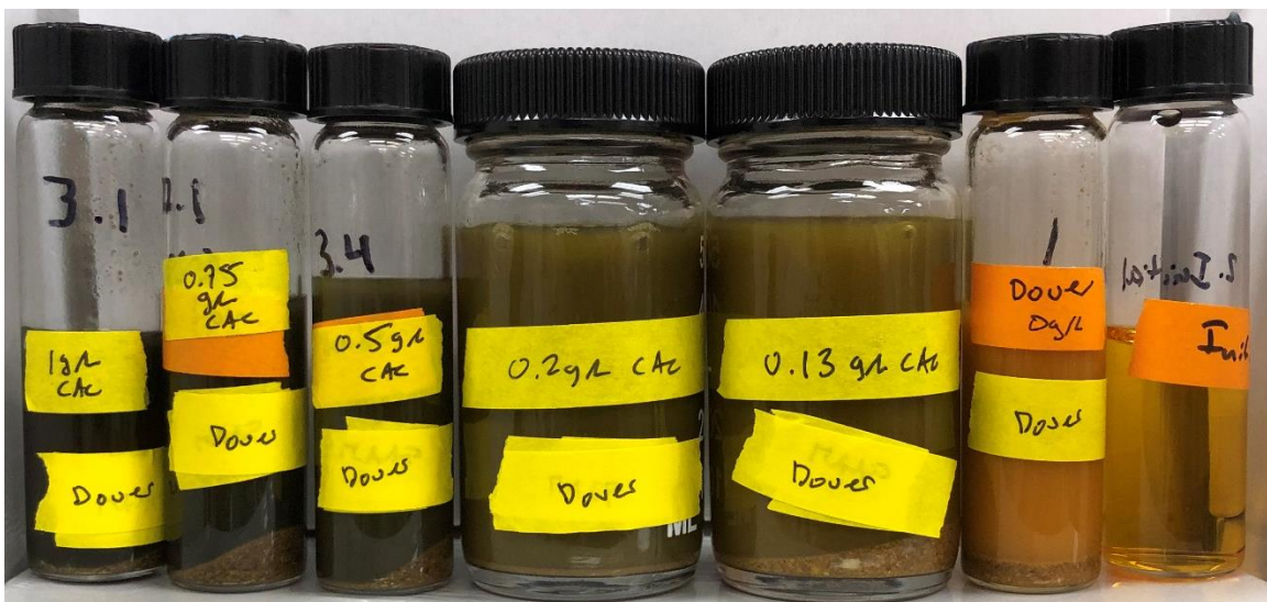
Figure 3.18- An image of the vials used in an experiment with polymer-free CAC-spiked Dover
