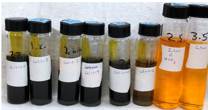
Figure 3.27- An image of the vials used in the tracer analysis of validation set 1, Column 1 samples. All vials contained 100 mg/L Orange G, 100 mM HCOOH, 100 mM HCOONa, and 100 g/L of a validation sample. The vials were labelled with the sample number (e.g., on the far left, Col-1-1). The pH of the solutions in the vials was between 3.6 – 3.7. The first 6 samples from the left contained validation set 1, Column 1 samples, while the 2 vials on the right were control vials, and as such did not contain soil. From left to right: samples Col-1-1, Col-1-2-, Col-1-3, Col-1-4, Col-1-5, Col-1-6, and two control vials.
