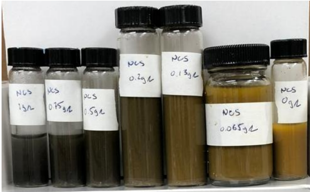
Figure 3.19- An image of the vials used in an experiment with PlumeStop®-spiked NCS
