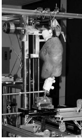
Figure 7: Example of a custom-built testing simulator from Driscoll et al. (2012). Custom simulator is shown with a mounted knee specimen. Adapted from [14].
