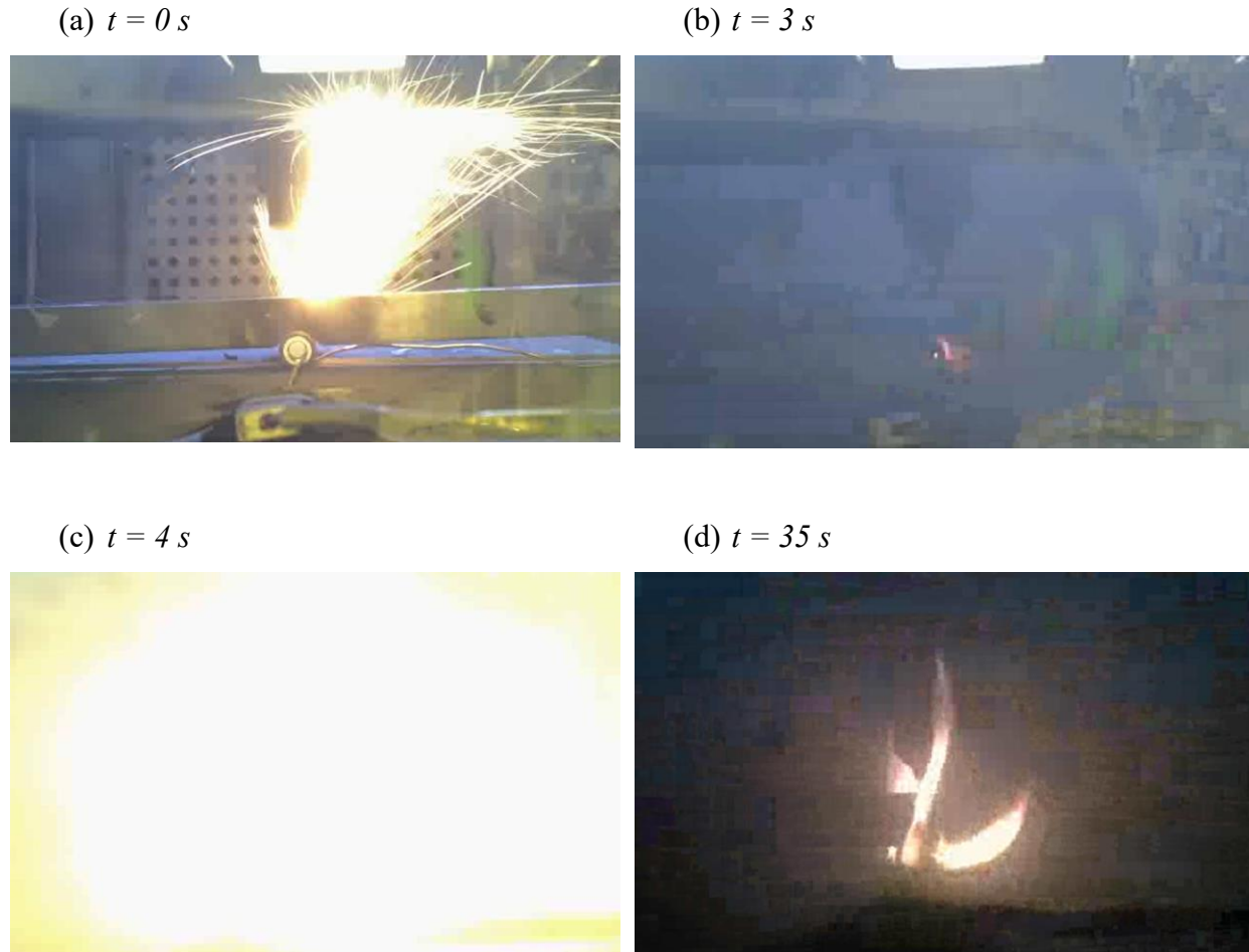
Figure 23: (a), (b), (c), (d) Progression of NP-induced TR in an LG-HG2 cell preconditioned to -40\text{ }^{\circ}\text{C} (Run 2). TR was initiated immediately following penetration, producing flaming ejecta from the penetration site
