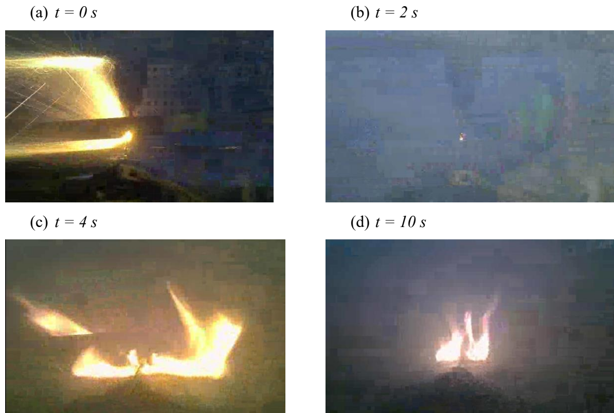
Figure 9: Progression of NP-induced TR in an LG-HG2 cell at 95% SOC. Following the (a) initial ejecta phase, (b) a brief pause in visible combustion was observed before the onset of (c), (d) secondary flame
