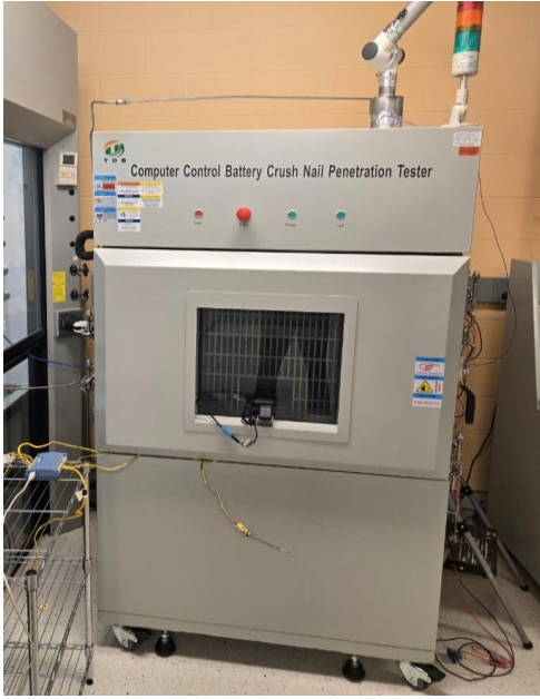
Figure 4: (a) TOB 6047 battery crush and nail penetration tester, (b) Explosion-proof chamber used for NP-induced TR experiments on lithium-ion cells
