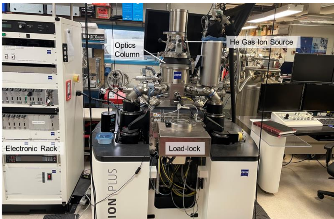
Figure 2.6 Photograph of the Orion plus helium ion microscope. Equipped with the integrated Nano-patterning and Visualization Engine (NPVE) by Fibics Inc., this HIM can also be used to perform helium ion beam lithography for nanodevice fabrication.
