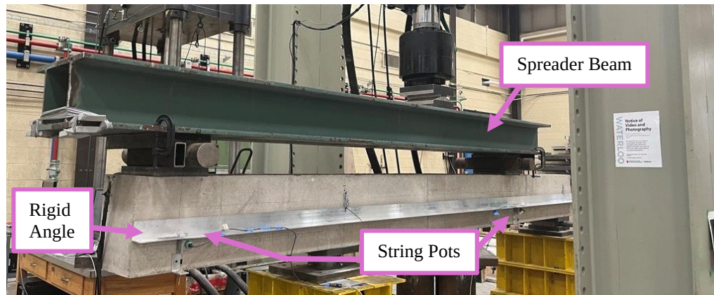
Figure 3.28. Displacement Measurement Mechanism
