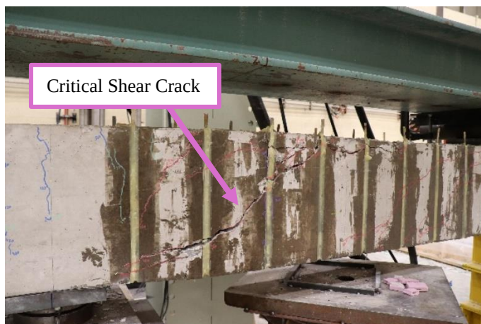
(a) Shear Failure
