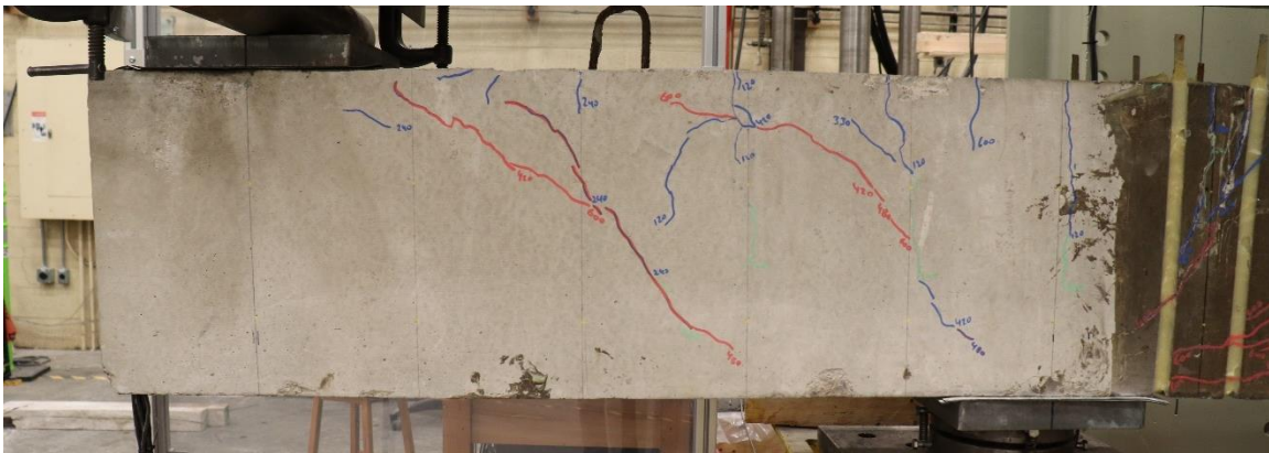
Figure A.14. Specimen A-100S-180C: Left Section (Transfer Span)
