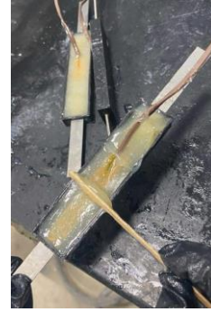
(b) Epoxy Composite Preparation
