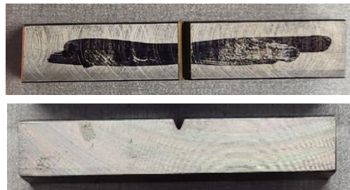
Figure 24: Charpy Impact (CVN) test specimen (with black marker on face with notch to indicate specimen orientation in testing machine)
