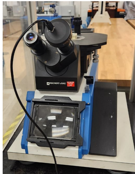
Figure 49: Reichert Jung MeF3 microscope used for microstructural observations
