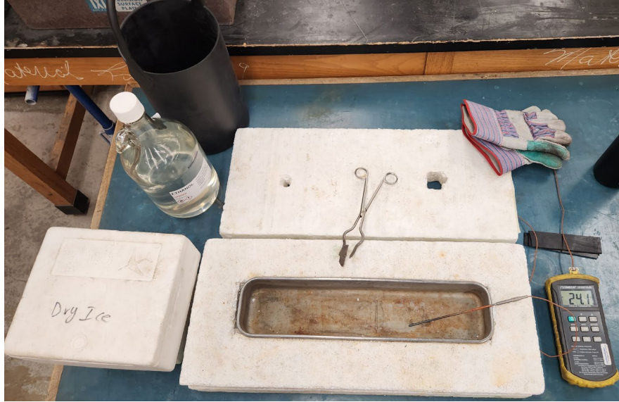
Figure 25: Charpy V-notch temperature control setup
