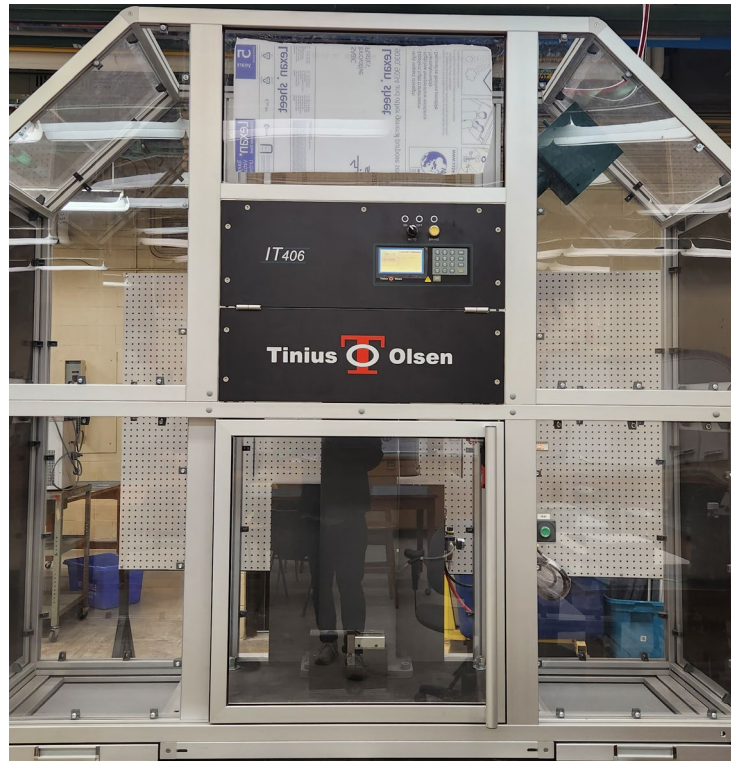
Figure 23: Tinius Olsen model IT406 pendulum impact tester for Charpy V-notch tests
